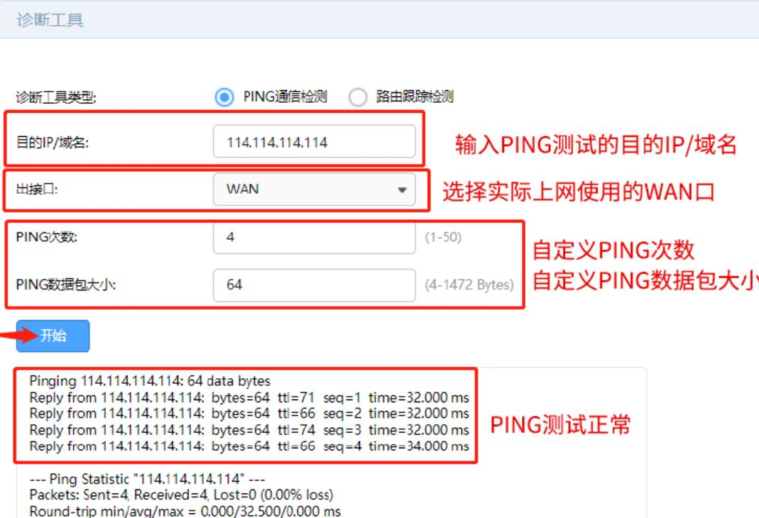
The screenshot shows the '诊断工具' (Diagnostic Tools) configuration page. It features a 'PING 通信检测' (PING Communication Detection) radio button selected. The configuration fields are as follows:
